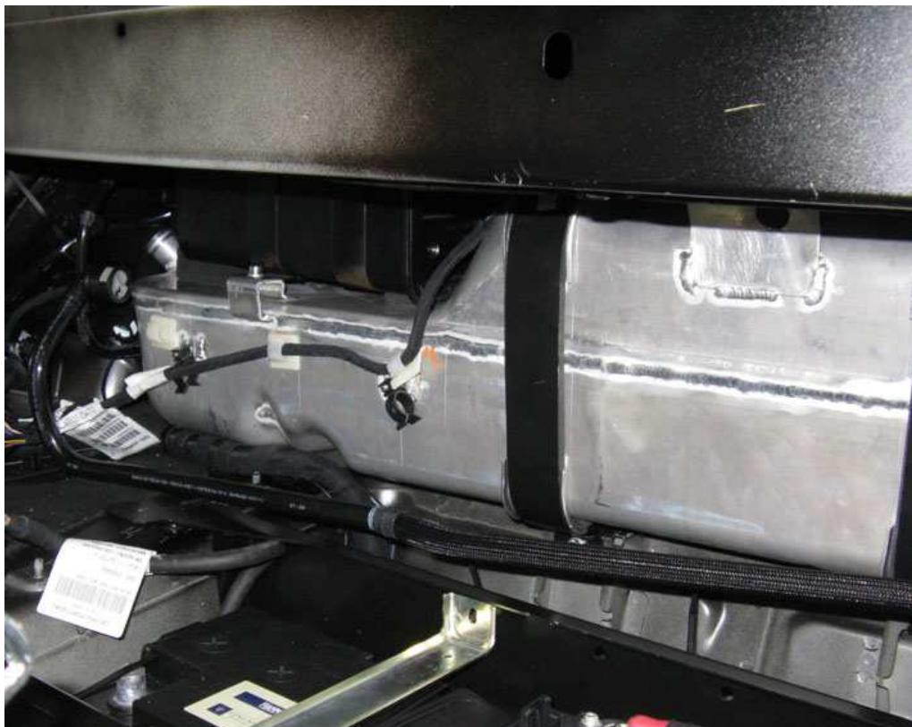
17. Unscrew the fastening nuts and move the complete battery mounting bracket towards the rear of the luggage compartment.
