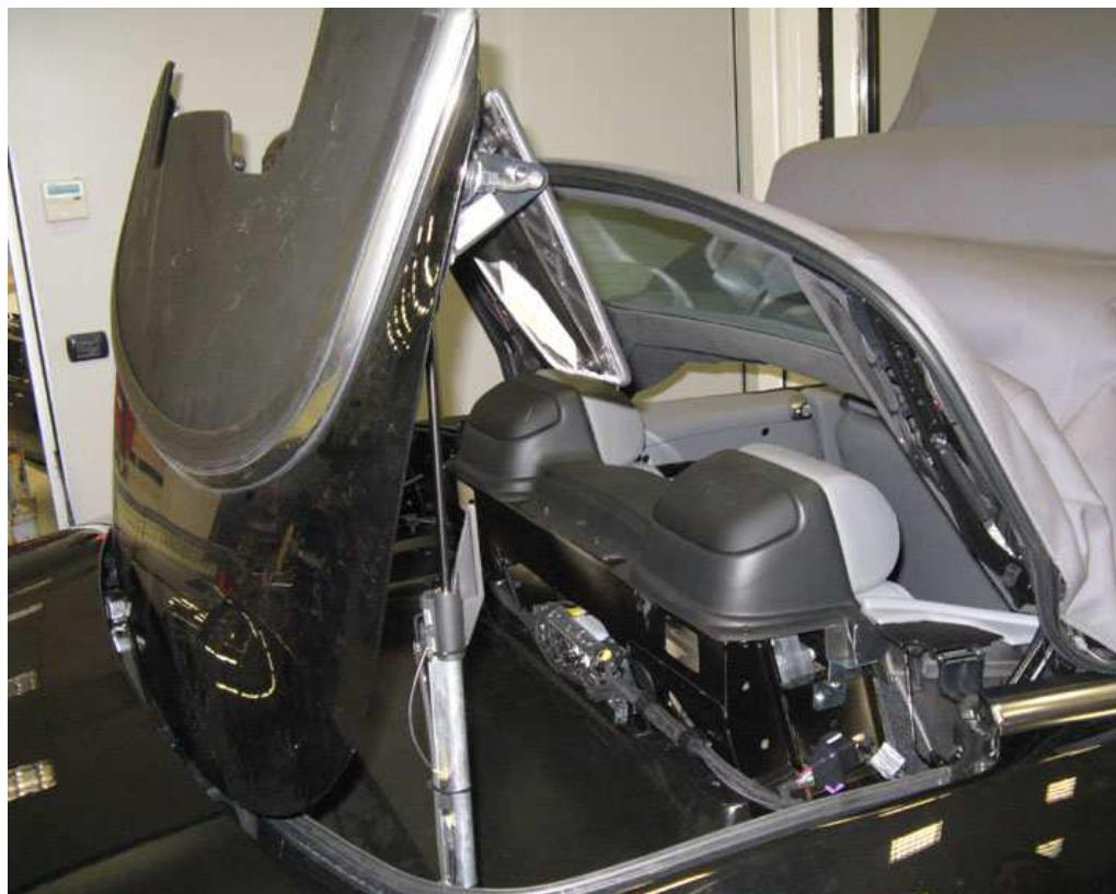
4. Block the Tonneau Cover using the tool 900028041, positioning the tool in line with the left-hand Tonneau Cover lock (1) and the left-hand Tonneau Cover striker plate (2).
