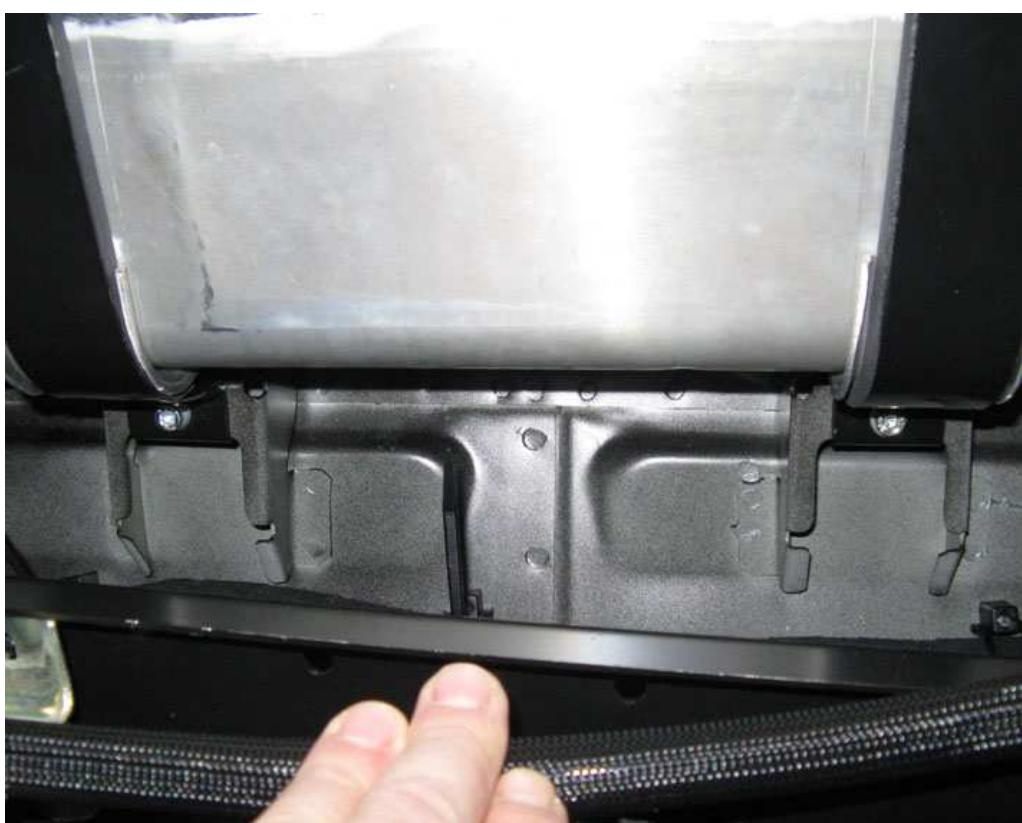
20. Remove the two fuel tank fastening brackets.
