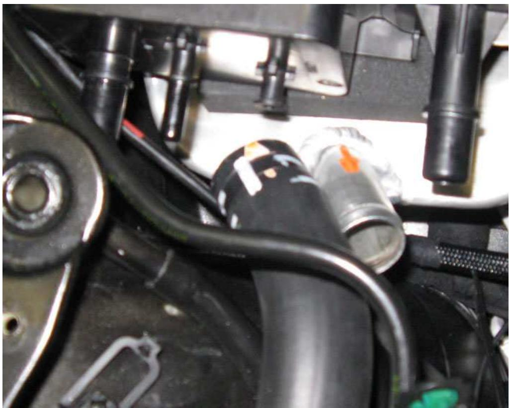
7. Open the fuel tank door, move the cap away and undo the screws (1) that secure the filler neck to the bodywork.
