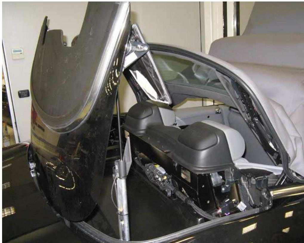
3. Block the Tonneau Cover using the tool 900028041, positioning the tool in line with the left-hand Tonneau Cover lock (1) and the left-hand Tonneau Cover striker plate (2).
