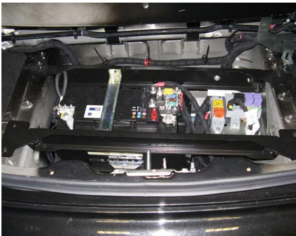
18. Detach the electrical connector for the fuel tank wiring.
